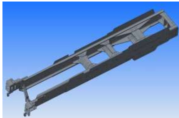
Flexible frame, bolt-on structure (Tonly, LGMG, Sany, SINO and other wide-body vehicles)
