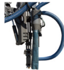
Cyclone Improves the life of the dust filters and increases the efficiency of the dust-control system by separating the larger pieces of aggregate at the front of the drill.
