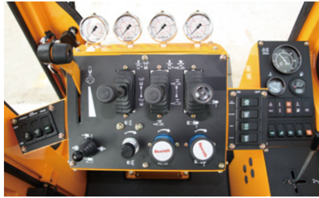
Operation Panel Drilling operation features a pilot hydraulic control system. This simple and efficient system eliminates any potential electrical problems in the drilling circuit.
