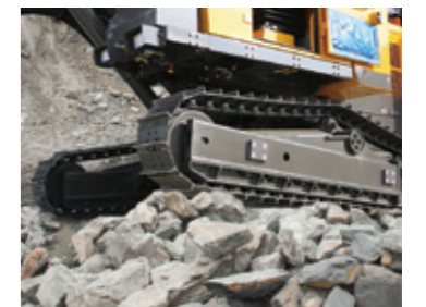
Oscillation Independent track oscillation provides safe, smooth and efficient mobility in rough terrain.
