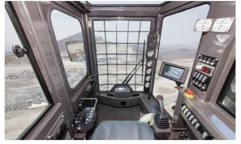
ROPS & FOPS certified cabin with accessible controls provides comfortable driving and easy operation. Indicators and gauges are located in the line of sight of the operator for good visibility
