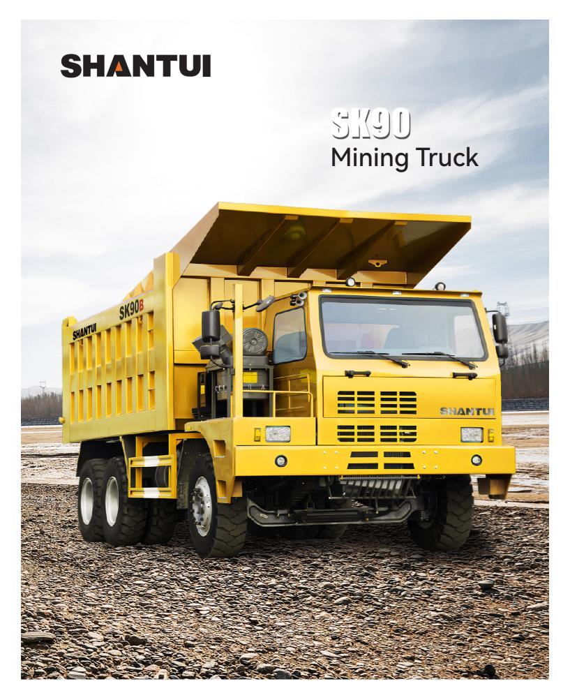
Engine model: Weichai WP12.430E201/WP12G460E470 Power/Speed: 316/1900kW/ rpm; 338/2100 kW/ rpm
