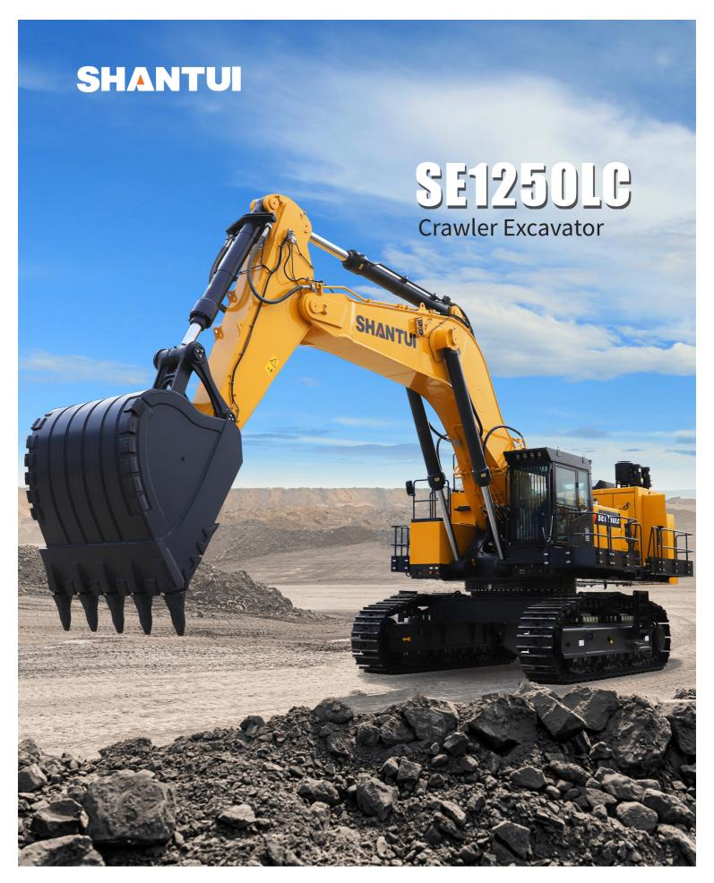
Engine Model: Gross Power: Operating Weight: Weichai 8M33 680 kW/1800 rpm 120,000kg
