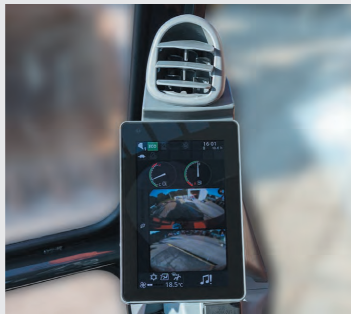
Low-reflective color 8" monitor, 42% larger display compared to ZX-5G series. Easier to view and navigate. Optional USB power supply and Bluetooth® available.
