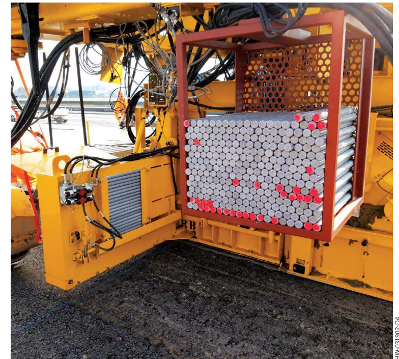
The hydraulic powered magazine-style side bar inserter allows personnel to load multiple bars into a magazine clip. The bar inserter then releases a single bar and places it at the specified distance.
