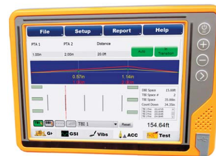
ACC (Accessories) Screen shows how many PTAs, TBIs, and SBIs are set up on the paver, and the distance between them.
