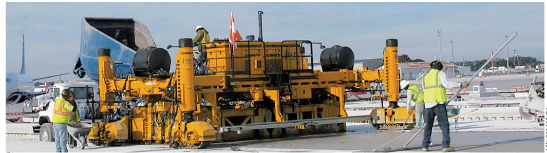
A GP-2400 featuring a 5400 series mold with two telescoping end sections, end slump adjustment, and a self-supported PTA paves a new airport ramp.
