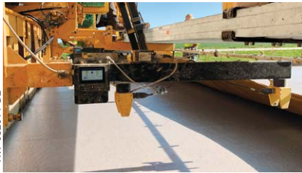
The LCD screens provide digital diagnostics at the sensor location or can send readouts to the optional Navigator system attached on the side of the paver.
