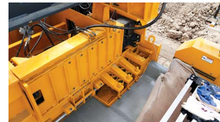
A GP-2400 featuring a 5400 series mold with two telescoping end sections, end slump adjustment, and a self-supported PTA paves a new airport ramp.
