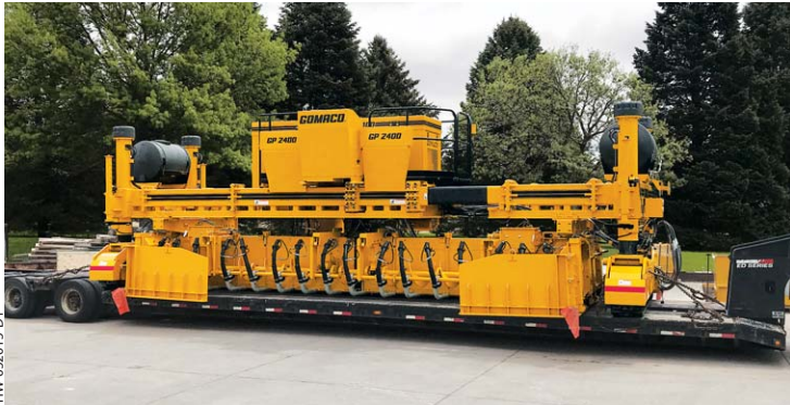
The two-track GP-2400 was designed for minimum transport width and for easy transportability between job sites.
