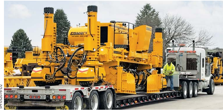
This four-track GP-2400 features optional rotary-sensored slew drives.
