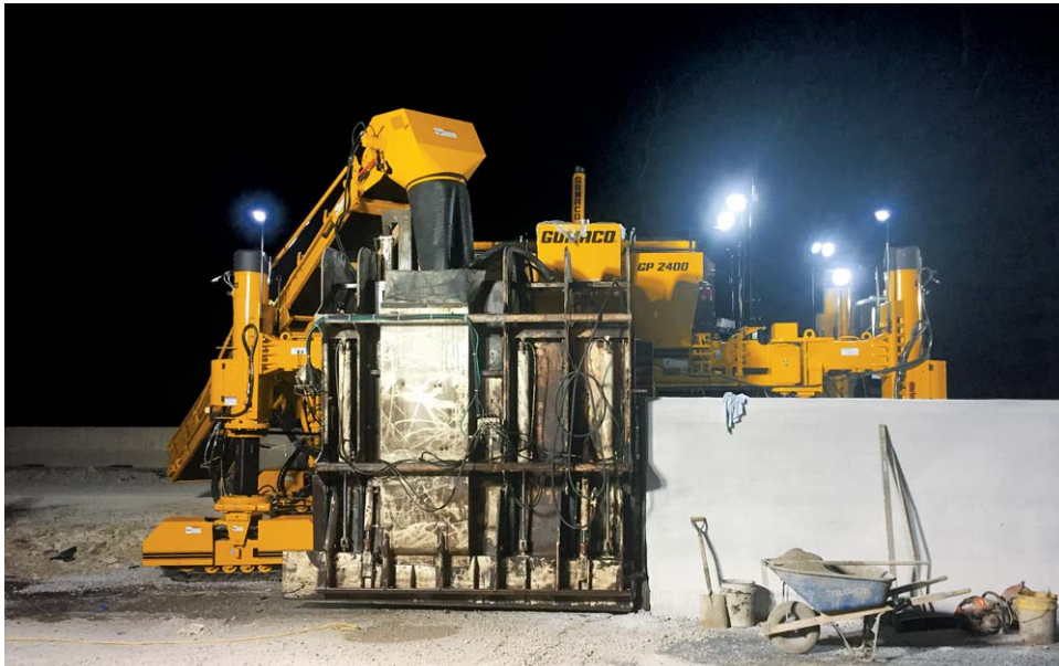
When transitioned into transport mode, the four-track GP-2400 is capable of slipforming barrier wall up to seven feet (2.13 m) tall.
