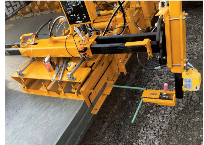
The two-track hydraulic powered bar inserter trails behind the mold and tracks.
