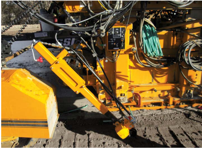
The four-track paver's hydraulic powered bar inserter is located in front of the rear paver leg at the end of the mold.
